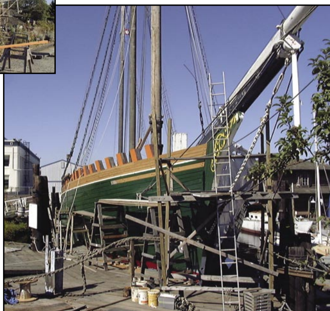
Left and Below: New planking on Wawona's bow.
