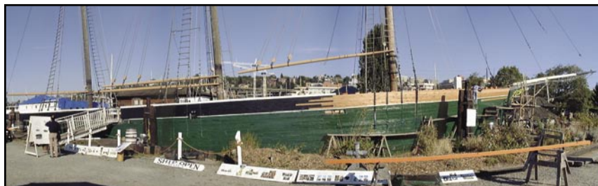
Left and Below: New planking on Wawona's bow.
